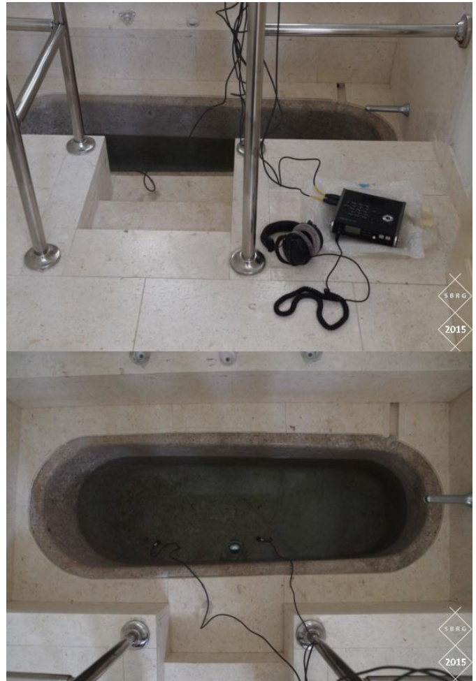
Figure 3. Top: the recording equipment Tascam DR-680 connected to the ultra-sensitive microphones. Bottom: the microphones (hydrophones) placed inside the tanks totally submerged in the water.
