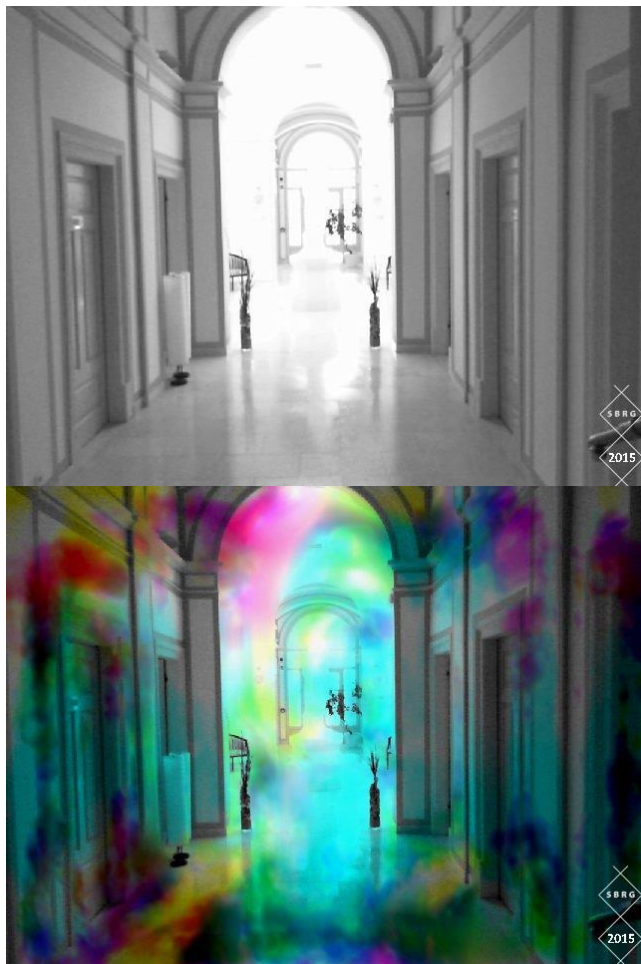
Figure 8. The same big room of Figure 6 taken from another angle in the visible band (above) and in UV band after TRV camera processing (below).
