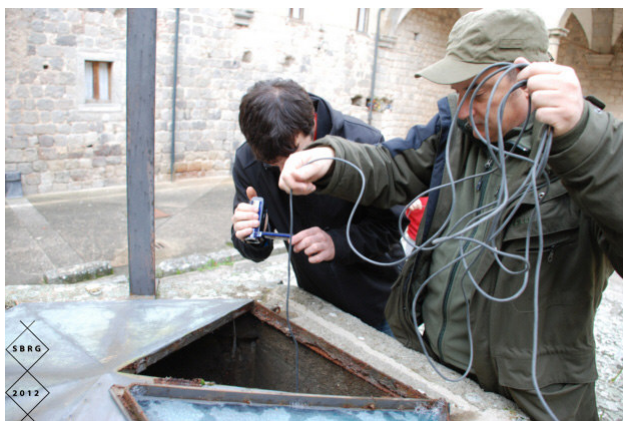
Fig. 4 - two microphones Hydrophones being placed in the well, despite a cable length of 12 meters, they did not resting on the bottom of the tank
