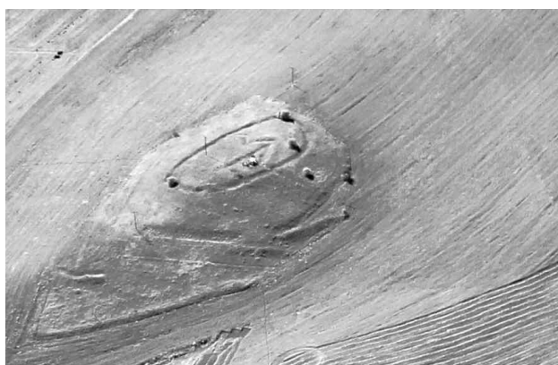
Figure 14. Aerial survey using an infrared camera: the vegetation is deleted by the photograph making more evident the different aspects of soil (photo: survey SBRG)
