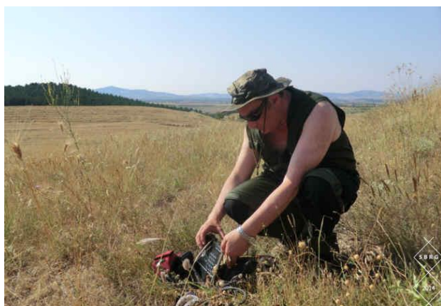
Figure 24. The portable digital recorder Tascam DR-680 during investigation placed on the ground, with the microphones inserted into the ground (photo: survey SBRG)
