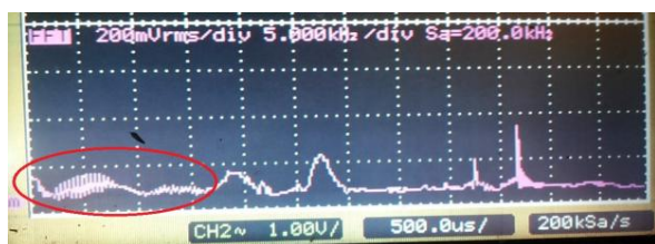
Figure 18. Signals in the range from 2 to 16 kHz with shape that are extremely peculiar and are correlated with the presence of water flows (photo: survey SBRG)
