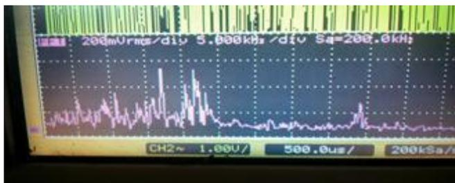
Figure 18. Spectrogram of electric field Sensor: rod antenna,  $l = 30$  cm, 5 kHz/div F [kHz]: 5, 9; 10.5; 12.; 14, 15, 16, 17; 20.5; 22; 23.5; 44
