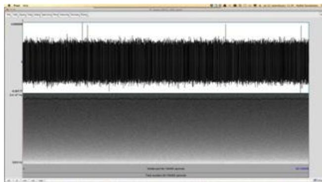
Figure 6a. Baseline 192kHz/16bit spectrum of the measuring system (viewed in Praat software).
