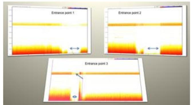
Figure 11. Small sensor data recorded while moving the directional small sensor above the presumed entrance point. The "hole" that's visible in the spectrums refers to a possible empty space (cavity) in the ground (x=frequency/Hz @ 192kHz sampling rate, y=time/secs). The same feature can be seen in the ~65kHz groundloop harmonic reference signal (BatSound software).
