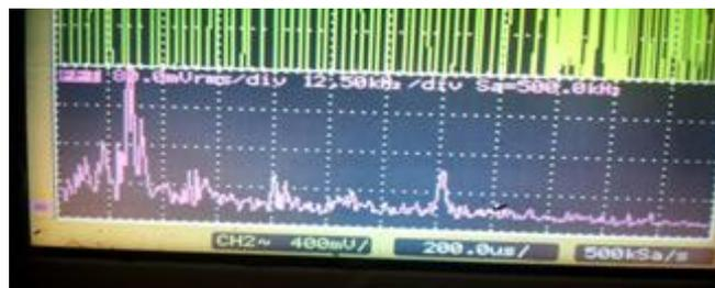
Figure 17. Spectrogram of electric field. Sensor: rod antenna, l = 30 cm, 12.5 kHz/div F [kHz]: 6.2; 11.2; 15; 17.5; 32.5; 51; 80; 87.5
