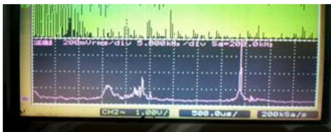
Figure 20. Sensor: open coil antenna, 5 kHz/div F [kHz]: 16; 23; 44.5;
