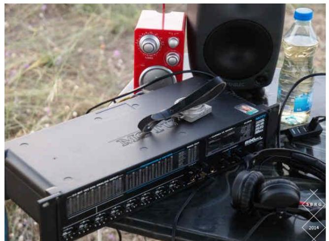
Figure 4. MOTU interface showing cables connected to the sensors and Genelec speakers to "sonify" the EM signals and mechanical waves being reflected from the tumulus
