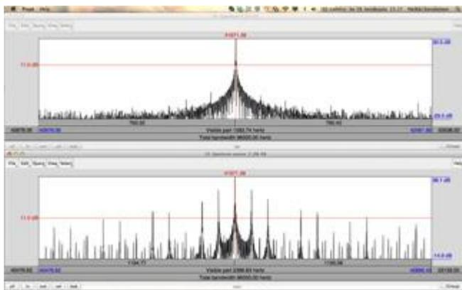
Figure 10b. Top Bylazora EM spectrogram zoomed in (42kHz peak). Bottom Geoglyph zoomed in scale. Visible part ~2kHz. Geoglyph seems to make harmonics of the ground loop signal.
