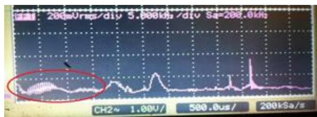
Figure 26. Signals in the range from 2 to 16 kHz with shape that are extremely peculiar and are correlated with the presence of water flow (photo: survey SBRG)
