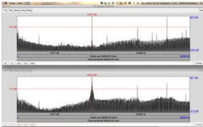
Figure 10a. Top Bylazora full range EM spectrogram, below the Geoglyph, the mound seems to amplify the groundloop signal (Praat software).
