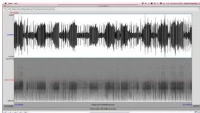
Figure 22. Zoomed (96kHz) ultrasound spectrogram recorded on top of the geoglyph (using a Pettersson D1000x bat detector). Typical natural sounds including insects exceed 50kHz. There are no ultrasound anomalies. Sampling rate 768kHz/16bit. Visible part 80 secs. Praat software.
