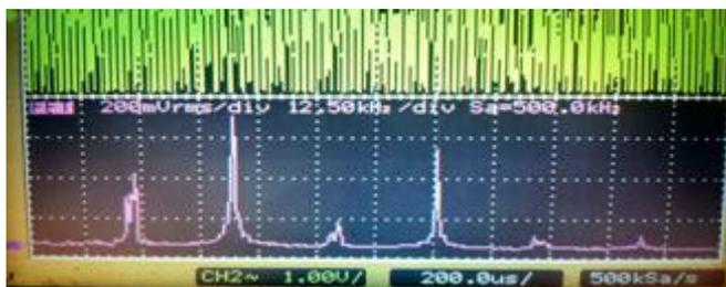
Figure 19. Sensor: open coil antenna, 12.5 kHz/div F [kHz]: 22.5; 45; 67.5; 87.5
