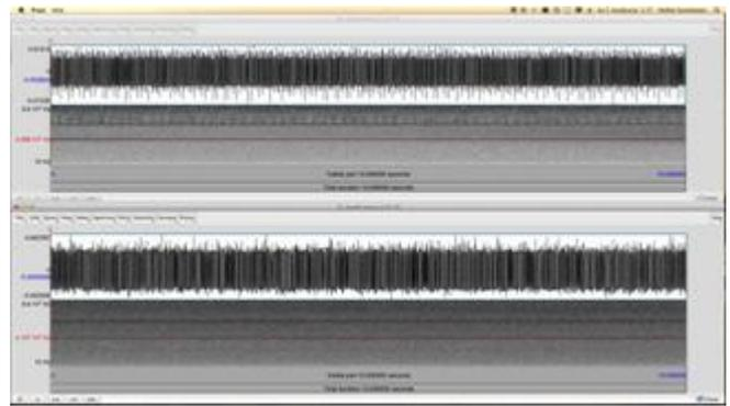
Figure 7. Comparative analysis. Bottom: Baseline X-angle EM spectrogram 700m north of Geoglyph mound. Top: same on top of the Geoglyph mound. The top results showed some interference & diffractions to the groundloop signal which are not found on the baseline results (Praat software).
