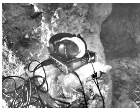
Fig. 6 – One of the digital recorders (Tascam DR-680) used during the audio analysis of Cividale del Friuli Hypogeum
