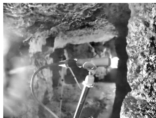
Fig. 7 - The high sensitivity Sennheiser MKH 3020 microphone
